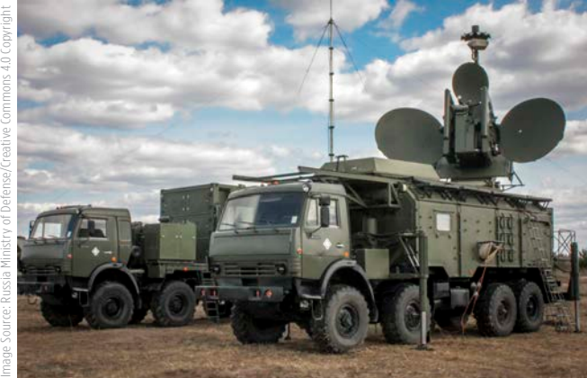
Russia has invested heavily in developing sophisticated electronic warfare capabilities, including this Krashuka-4 jammer.
