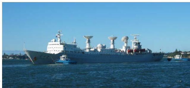
This Chinese Yuan Wang space tracking ship, which supports space launch operations from positions in the Pacific, is part of China’s SSA network. 115
